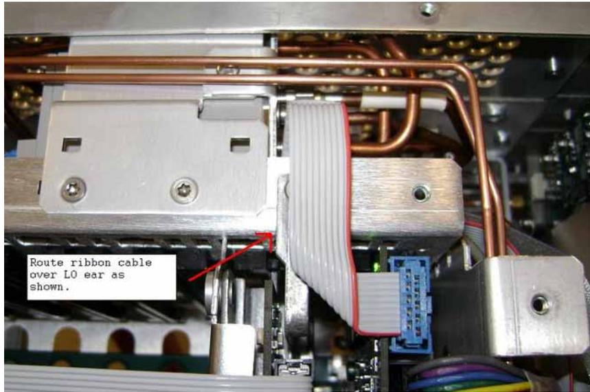
**Figure 16-36 Cable Routing**
